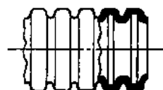
Coarse profile G High pull-out strength.
